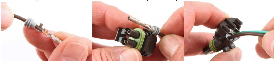
WIRE WITH TERMINAL AND SEAL ASSEMBLED INTO HOUSING
