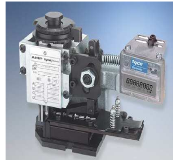
CRIMP TOOL WITH CYCLE COUNTER
