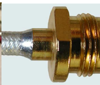
SOLDERED CONNECTOR
