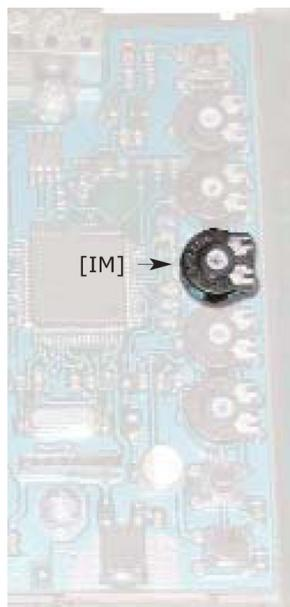
The reverse motion torque parameter sets the sensitivity degree to detect an obstacle during the door closure, thus giving the reopening command. The parameter's value can be manually set through the [IM] regulation trimmer (turning it clockwise will set the reversing system force from the minimum value to the maximum value)
