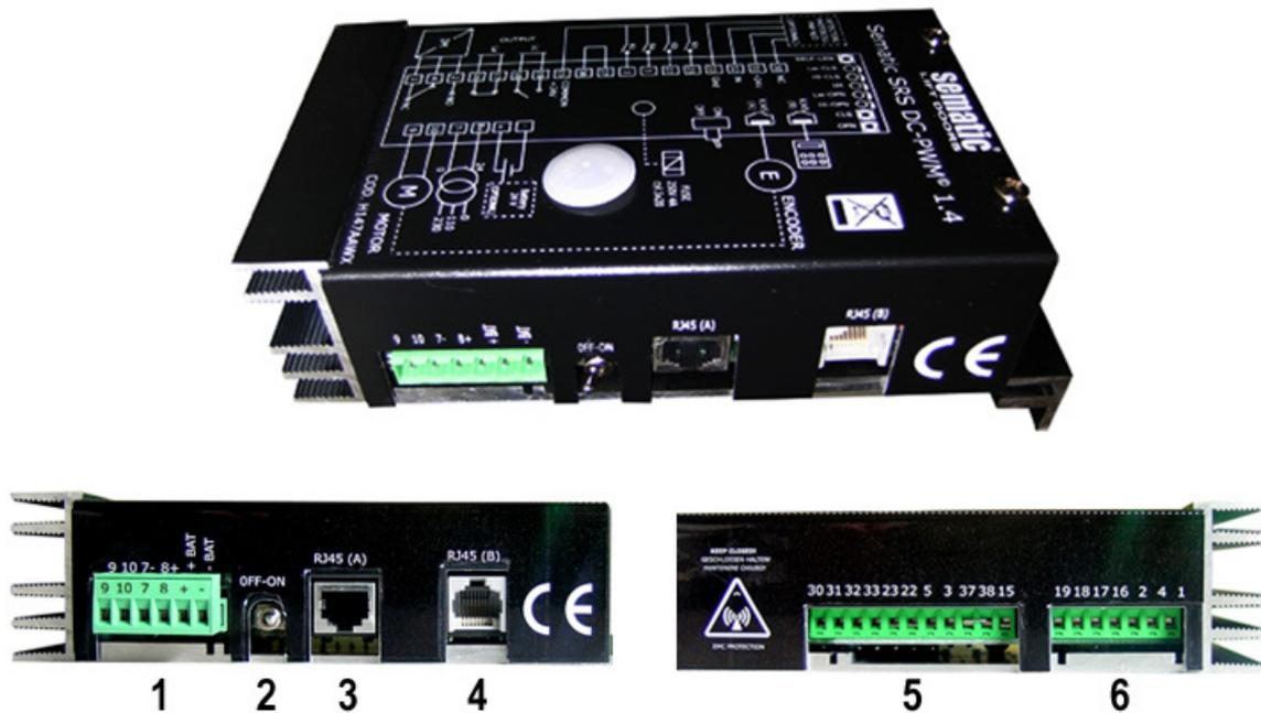
1. 6 poles connector for motor, 24 Vac power supply and auxiliary battery supply
