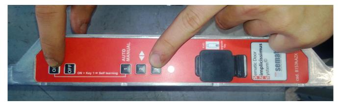
3. Keeping push key 3 (><), push also the key ON; after that release both keys.
