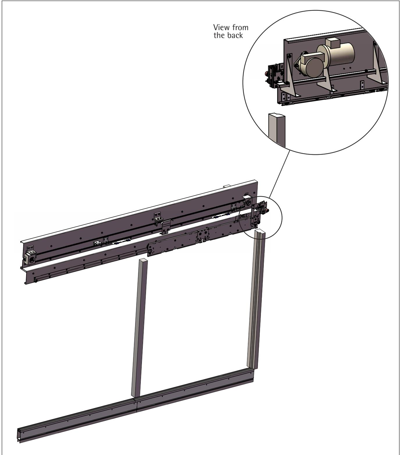
Fix the mechanism to the car, according to designed approved drawings.
