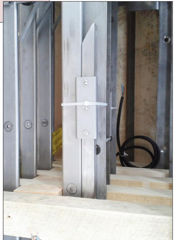
Disassembly the fix cam from the mechanism.
