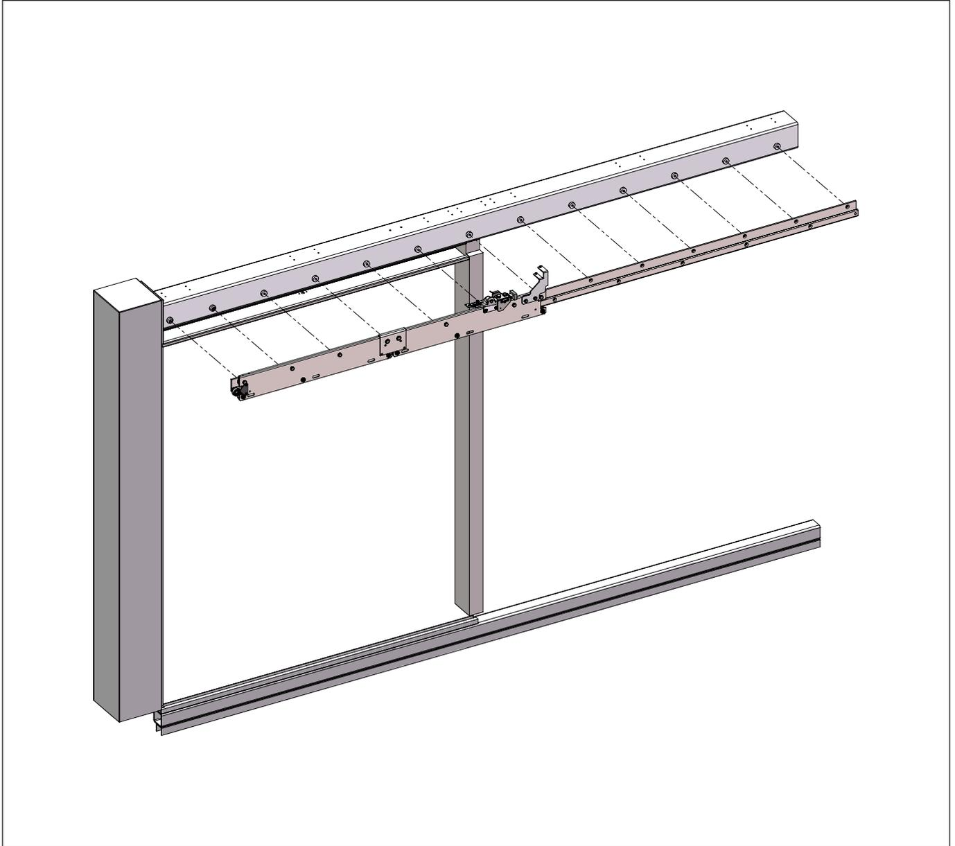
Fix the mechanism directly on the existing spacer, the spacers welded on the IPE profile.
